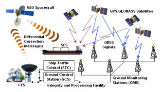
Figure 5. Maritime GASDL System for Enhanced GMDSS Network
