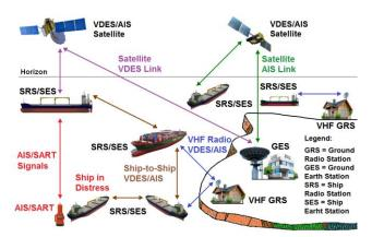
Figure 3. New Concept of VDES/AIS Network
