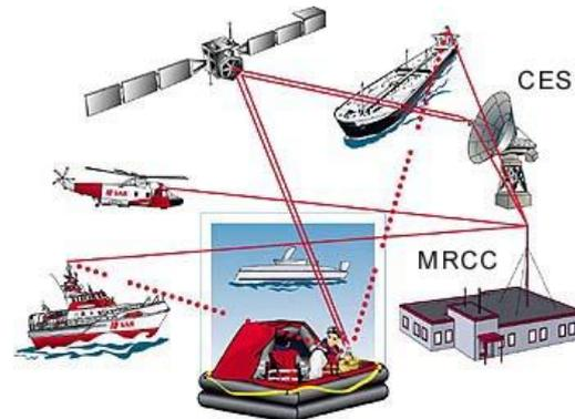
Fig.2. Inmarsat system communication.
