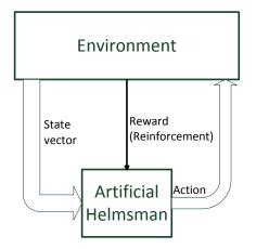
Figure 1. Interaction of helmsman with an environment.
