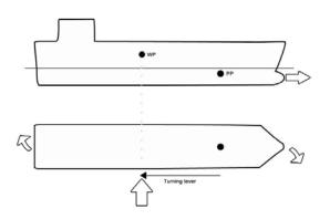
Figure 2. Wind effect and turning lever of ship mowing forward.
