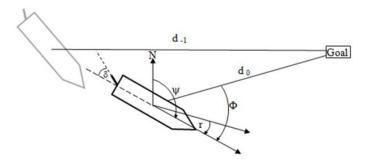
Navigational situation of a moving vessel can be described in many ways. Most important is to define proper state vector from abundant range of data signals (Fig. 6.) and arbitrary determine fitness function values received by the helmsman.
