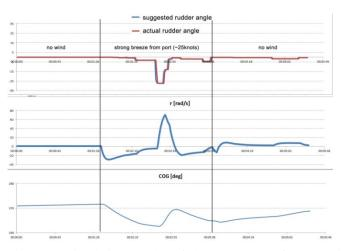
Figure 8. Simulation results of the systems performance in heavy wind environment.
