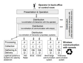
Figure 4. The processing communication and navigation information system in back-offices and the RIS control rooms management centres in the BICS standard [4.8].
