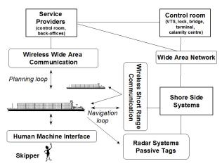
Figure 2. Processing and transmission navigation data in the RIS system [3]
