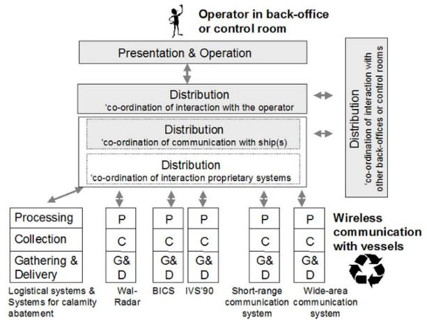
Figure 4. The processing communication and navigation information system in back-offices and the RIS control rooms management centres in the BICS standard [4.8].
