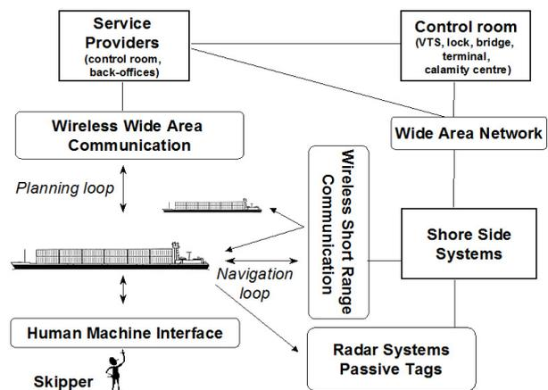
Figure 2. Processing and transmission navigation data in the RIS system [3]
