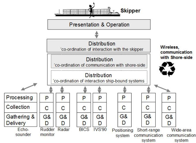
Figure 3. The data communication and information system on-board of a vessel in the BICS standard [4,8].
