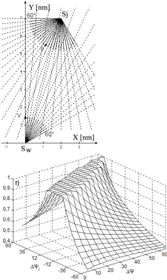
Figure 3. Met  $j$ -th ship on the starboard side: the sets of acceptable game strategies of own-ship  $S_w$  and  $j$ -th encountered ship  $S_j$  (above), and hyperplane of collision-risk  $r_j$  depending on the  $\Delta\psi$  own-ship course changes and the encountered  $j$ -th ship  $\Delta\psi_j$  (below).
