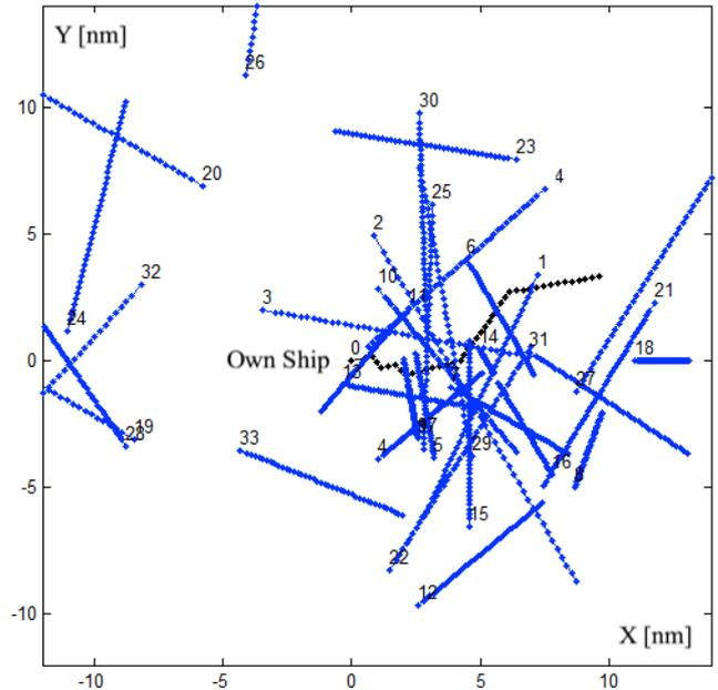
Figure 9. A safe trajectory of own-ship in non-co-operative matrix game, in conditions of restricted visibility of the sea, for  $D_s = 2.6$  nm,  $p_f = 2.18$  nm (nautical mile).
