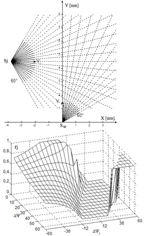
Figure 4. Met  $j$ -th ship on the port side: the sets of acceptable game strategies of own-ship  $S_w$  and  $j$ -th encountered ship  $S_j$  (above), and hyperplane of collision-risk  $r_j$  depending on the  $\Delta\psi$  own-ship course changes and the encountered  $j$ -th ship  $\Delta\psi_j$  (below).
