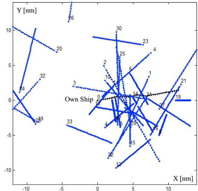
Figure 10. A safe trajectory of own-ship in co-operative matrix game, in conditions of good visibility in the sea, for  $D_s = 1.0$  nm,  $p_f = 0.57$  nm (nautical mile).
