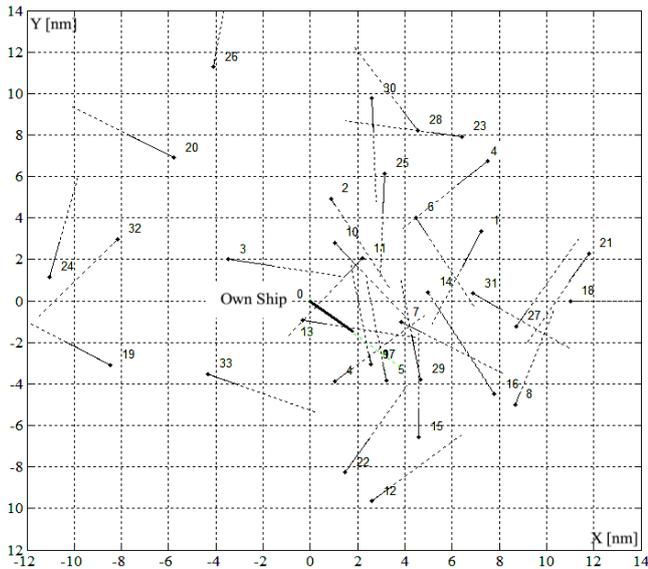
Figure 7. The six-minute speed vectors of own ship and 33 encountered ships in a navigational situation in Kattegat Strait.
