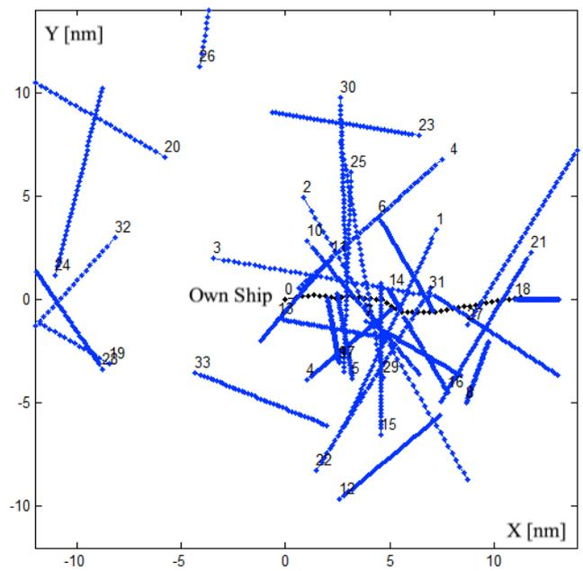
Figure 8. A safe trajectory of own-ship in non-co-operative matrix game, in conditions of good visibility in the sea, for  $D_s = 1.0$  nm, final payment  $p_f = 1.88$  nm (nautical mile).
