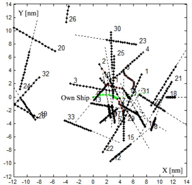
Figure 13. A safe trajectory of own-ship in non-game control, in conditions of restricted visibility on the sea, for  $D_s = 2.6$  nm,  $p_f = 0.71$  nm (nautical mile).
