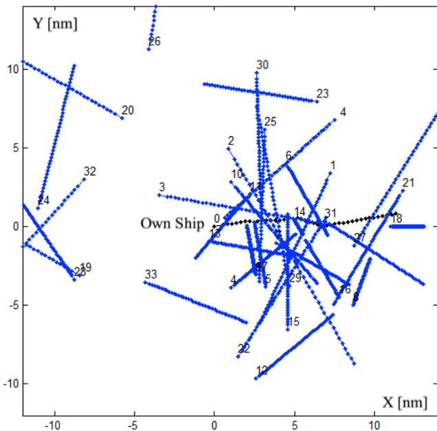
Figure 11. A safe trajectory of own-ship in co-operative matrix game, in conditions of restricted visibility of the sea, for  $D_s = 2.6$  nm,  $p_f = 1.19$  nm (nautical mile).
