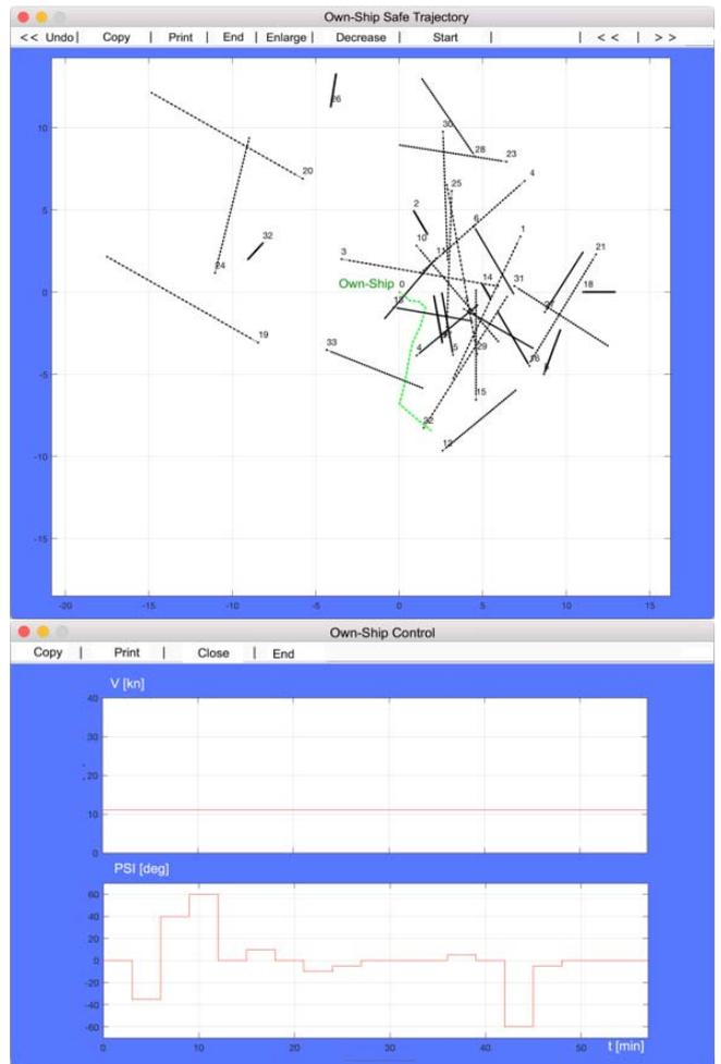
Figure 6. The algorithm window with the results of calculations of the safe own-ship trajectory and own-ship control by change of speed  $V$  or course  $\psi$ .
