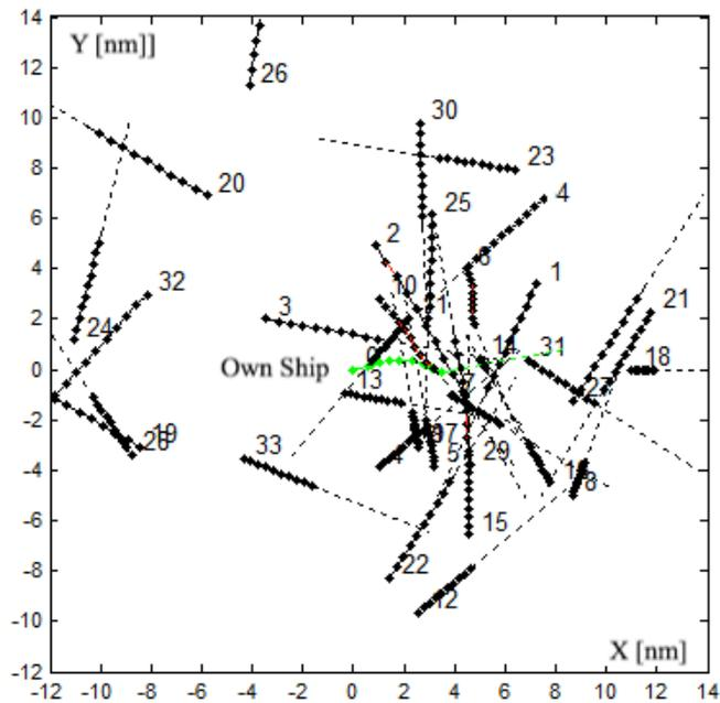
Figure 12. A safe trajectory of own-ship in non-game control, in conditions of good visibility on the sea, for  $D_s = 2.6$  nm,  $p_f = 0.69$  nm (nautical mile).
