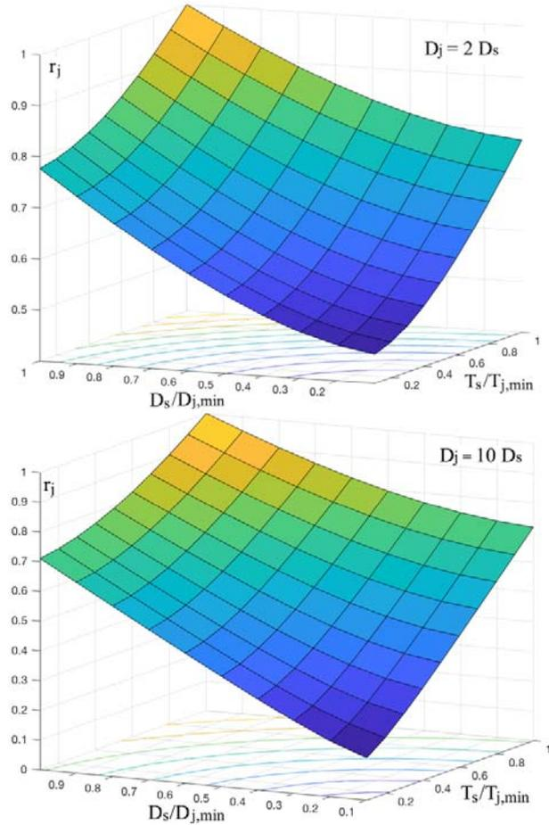
Figure 2. Collision-risk characteristics in the situation of concentrated ship traffic at:  $a_1 = a_2 = 0.4$ ,  $D_s/D_j = 0.5$  (above) and in the situation of larger distances between ships at:  $a_1 = a_2 = 0.5$ ,  $D_s/D_j = 0.1$  (below).
