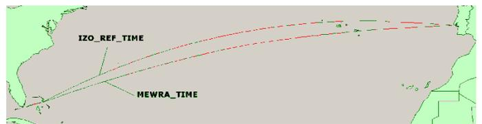
Figure 6. Output of the algorithm MEWRA\_TIME compared to the time-optimal isochrone route for Lisbon-Miami voyage, departure 2008-09-02 00:00
