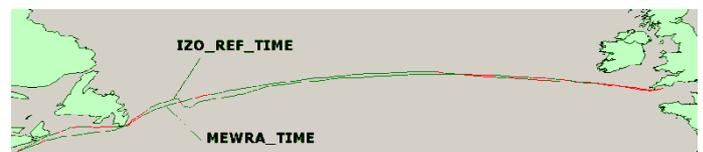
Figure 12. Output of the algorithm MEWRA\_TIME compared to the time-optimal isochrone route for Halifax - Plymouth voyage, departure 2008-02-15 12:00
