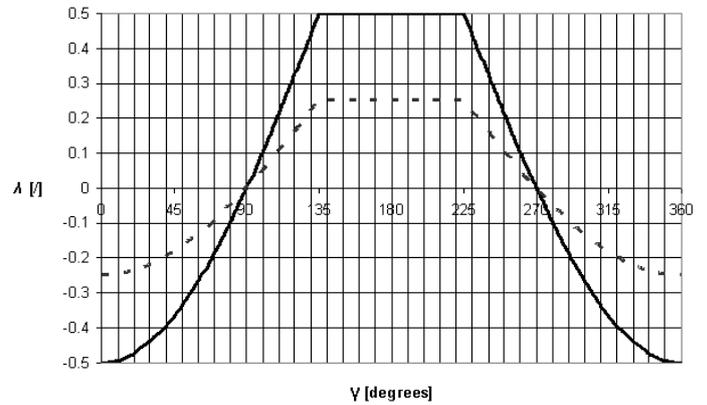
Figure 2.  $\lambda$  shape coefficient (solid line - hybrid propulsion; dotted line - only motor engine) as a function of wind heading angle  $\gamma$
