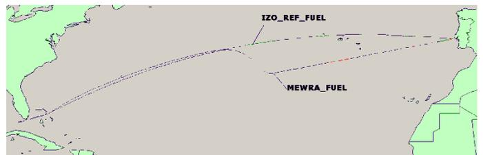
Figure 7. Output of the algorithm MEWRA\_FUEL compared to the fuel-optimal isochrone route for Lisbon-Miami voyage, departure 2008-09-02 00:00
