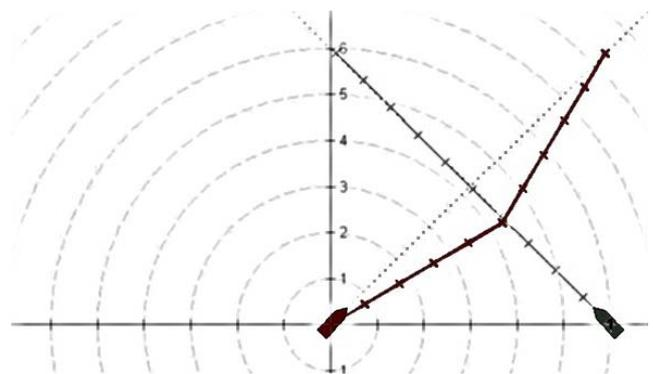
Figure 2. The optimal trajectory for avoiding a dangerous object that crosses the ship's course at right angles.
