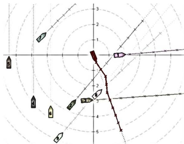
Figure 3. The ship optimal safe trajectory in passing with 9 objects.
