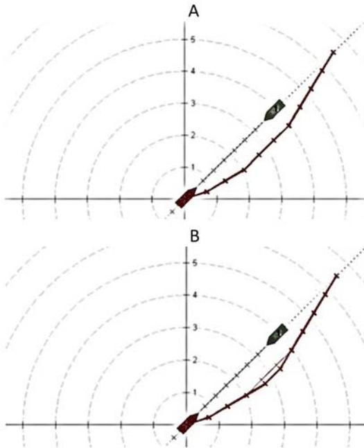
Figure 1. Comparison of trajectories with good and bad visibility in the case of ships heading straight towards each other, A - f good visibility, B - limited visibility.
