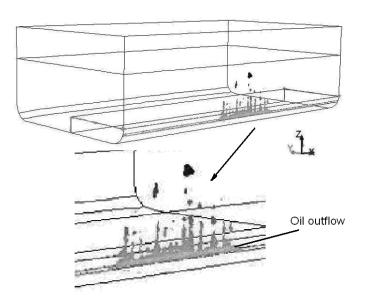
Figure 8. A typical flow pattern obtained for bunker oil outflow by the use of CFD simulations
