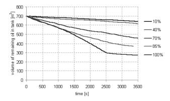
Figure 10. The volume of remaining oil in a damaged bunker tank (the initial volume of full tank was equal 700 m<sup>3</sup>)
