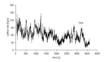
Figure 12. The rate of an oil outflow for the length of damage equal to 70% of considered section's length
