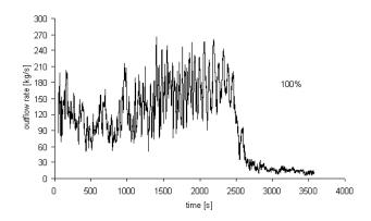
Figure 14. The rate of an oil outflow for the length of damage equal to 100% of considered section's length
