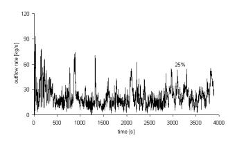
Figure 11. The rate of an oil outflow for the length of damage equal to 25% of considered section's length
