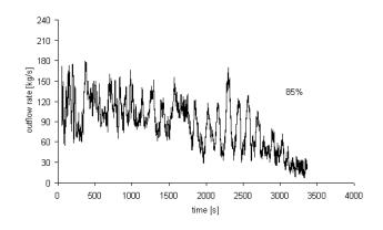
Figure 13. The rate of an oil outflow for the length of damage equal to 85% of considered section's length
