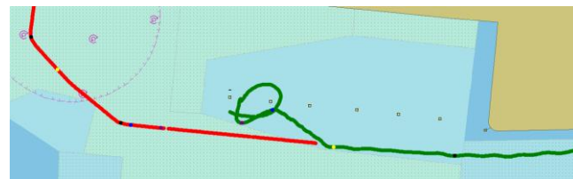
Figure 6. Driven Tracks in Scenario 2. The red dots represent the track of the target ship, while the green dots represent the real-world ownship. The yellow, blue and purple points represent the position of the real-world ownship and the simulated target ship at the same time on key positions. (Professional+ chart data from Lloyd's Register/i4Insight in a ChartServer solution from ChartWorld).
