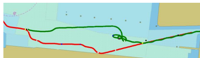
Figure 7. Driven Tracks in Scenario 3. The red dots represent the track of the target ship, while the green dots represent the real-world ownship. The yellow, blue, purple and white points represent the position of the real-world ownship and the simulated target ship at the same time on key positions. (Professional+ chart data from Lloyd's Register/i4Insight in a ChartServer solution from ChartWorld).
