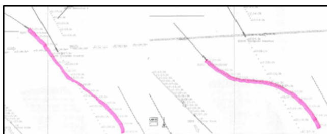
Figure 6. Samples of scenario track records for remote control of an unmanned ship, having available full bridge equipment in the SCC (left team 'no seafaring experience'; right: team with seafaring experience)
