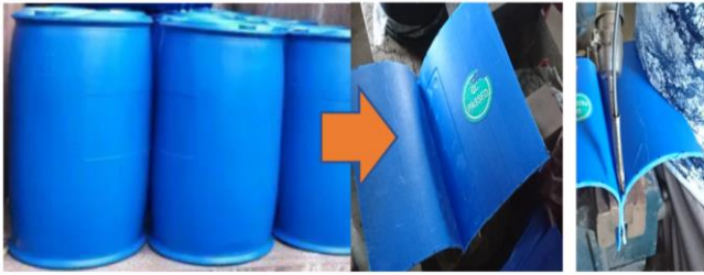
(a) HDPE blue drum scarp (b) Joining two layers of HDPE sheet by welding Figure 2. Joining two layers of HDPE sheet by HDPE welding
