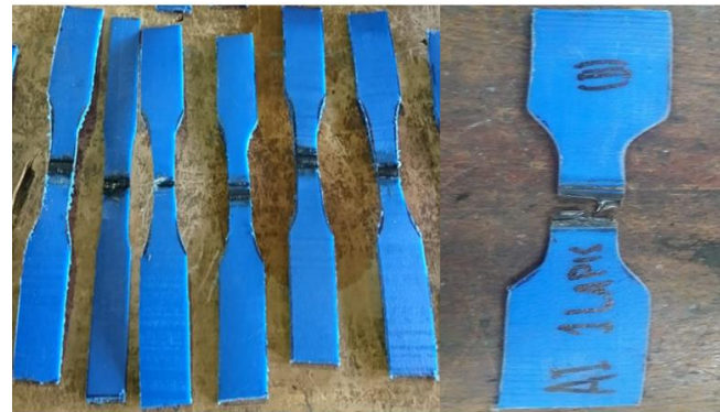
Figure 12. (a) Tensile test sample; (b) tensile test results
