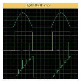
Figure 8. The operation oscillograms of a three-phase voltage sensor with digital integration and synchronization with the network
