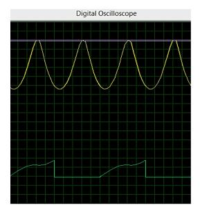
Figure 6. Oscillograms of the voltage sensor of a three-phase network when two phases are disconnected (single-phase mode)
