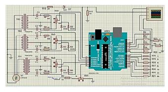
Figure 7. Circuit of a three-phase voltage sensor with digital integration and formation of a synchronization pulse
