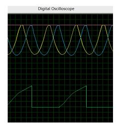
Figure 5. Oscillograms of the voltage sensor of a three-phase network when one of the phases is disconnected
