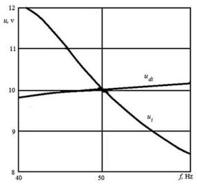
Figure 1. Dependence of the output signal of the AC voltage sensor on the current frequency:  $u_i$  – integration of the rectified voltage;  $u_{di}$  – preliminary differentiation, rectification, and integration of voltage
