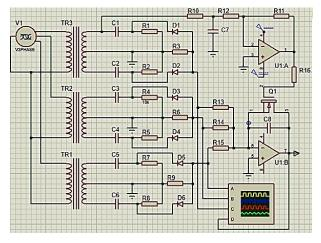
Figure 2. Analog part of the sensor for the average voltage of a three-phase network
