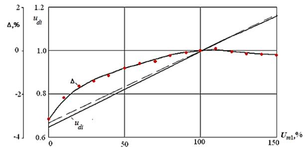
Figure 4. Accuracy and error in measuring the average value of asymmetric phase voltages
