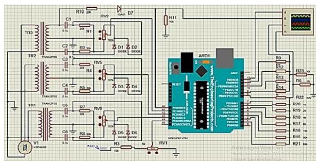
Figure 7. Circuit of a three-phase voltage sensor with digital integration and formation of a synchronization pulse
