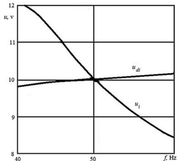
Figure 1. Dependence of the output signal of the AC voltage sensor on the current frequency:  $u_i$  – integration of the rectified voltage;  $u_{di}$  – preliminary differentiation, rectification, and integration of voltage
