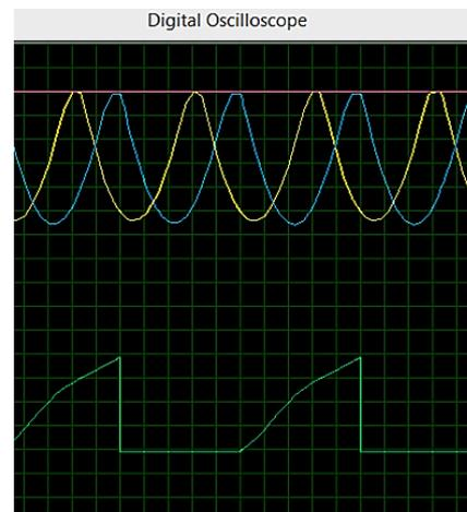
Figure 5. Oscillograms of the voltage sensor of a three-phase network when one of the phases is disconnected
