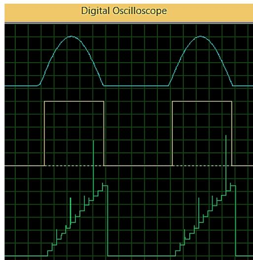
Figure 8. The operation oscillograms of a three-phase voltage sensor with digital integration and synchronization with the network
