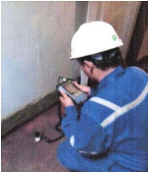
Figure 1. Ship vibration measurement
