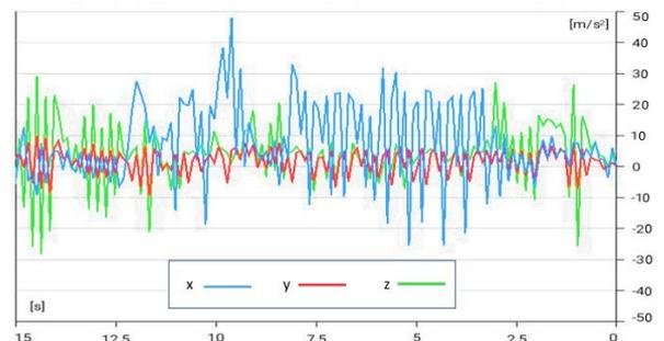
Figure 5. Vibrations before adding a side deck girder
