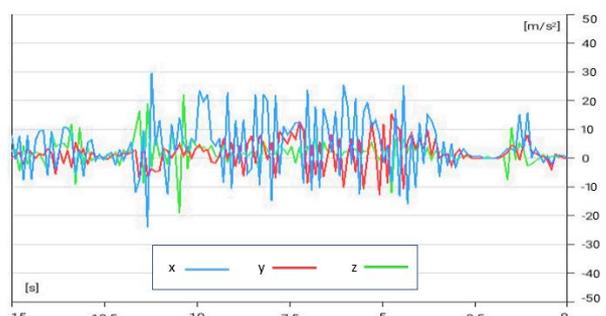
Figure 6. Vibrations after adding a side deck girder
