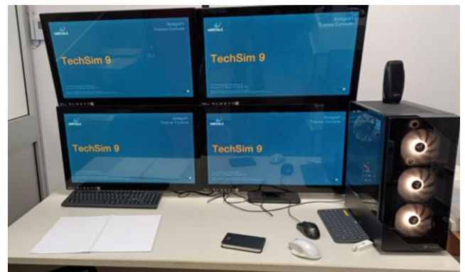
Figure 5. The trainee station of the engine room simulator at UNIGE
