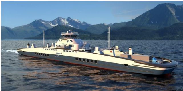
Figure 3. Double-ended ferry – HAV Design, double-ended design H-936.
