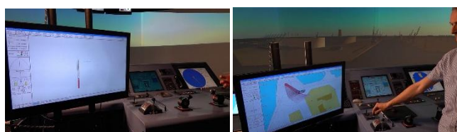
Figure 7. SAMMON Monitoring & Conning Tool with Multiple predictions used in Ship Handling Simulator for Training used in familiarisation exercise for Podded Ships
