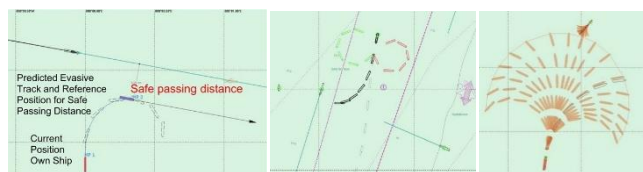
Figure 9. Visualising lower action limit for "Stand on Vessel" (left), multiple prediction of maximum manoeuvres (centre) and manoeuvring zones with all potential manoeuvres (right)
