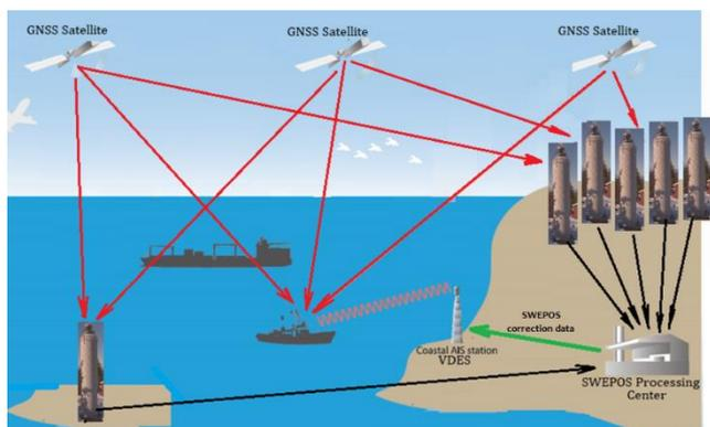
Figure 4. Dissemination of GNSS correction data via VHF and VDES.
