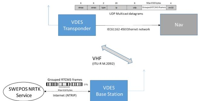
Figure 5. Transfer of GNSS NRTK corrections via VDES.
