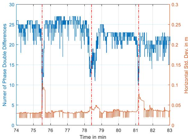
Figure 17. Number of double difference carrier phase measurements and horizontal positioning accuracy during three passages below bridges.
