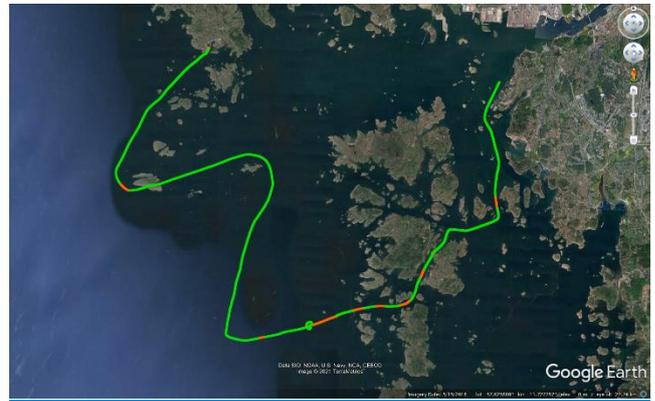
Figure 13. Shipping route of 2 hours in Gothenburg area. The color denotes the availability of a fixed RTK solution, i.e. green sections refer to a fixed RTK solution and red sections refer to a float RTK solution.
