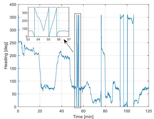
Figure 14. Heading solution over time. The enlarged section shows the variation of heading during some turns.
