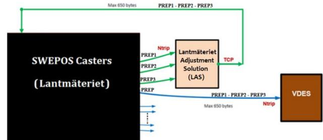
Figure 6. Data flow of GNSS correction data before dissemination via internet and VHF
