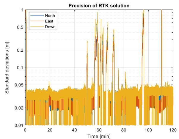
Figure 15. Precision of RTK solution over time during 2 hour shipping route: The precision is better than 5 cm for a fixed RTK solution, and degrades to a few decimeters for a float RTK solution. A fixed solution is obtained for most of the time. Position accuracy when performing the maneuver.
