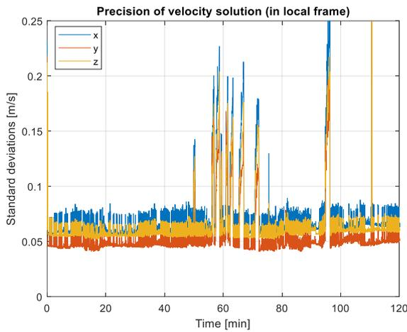
Figure 16. Precision of 3D velocity solution in local vessel coordinate frame over time. The precision varies between 5 cm/s and 8 cm/s for a fixed RTK solution and degrades to 25 cm/s for a float RTK solution.
