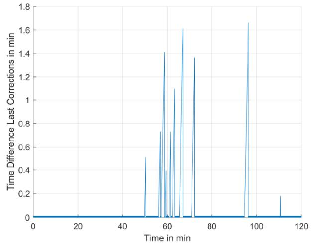
Figure 18. Outages of the RTK correction data.
