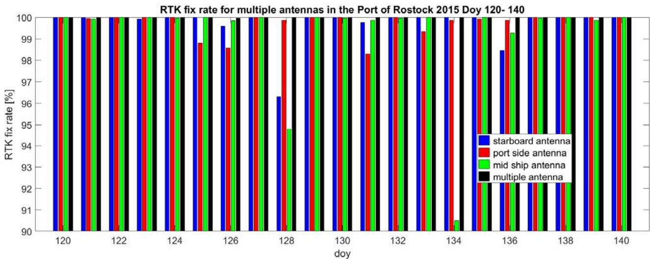
Figure 11. RTK fix rate for multiple antennas in the port of Rostock
