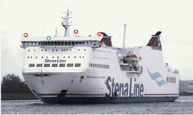
Figure 3. Vessel Mecklenburg-Vorpommern with positions of the GNSS antennas (red circles) and location of the board with receivers (green circle)
