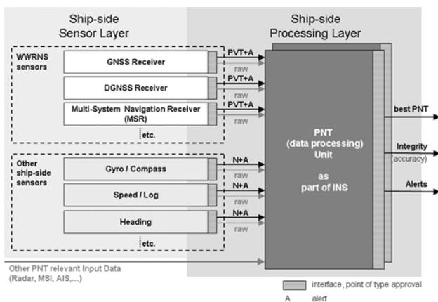
Figure 1. Concept of a PNT data processing Unit as part of a future Integrated Navigation System (INS)
