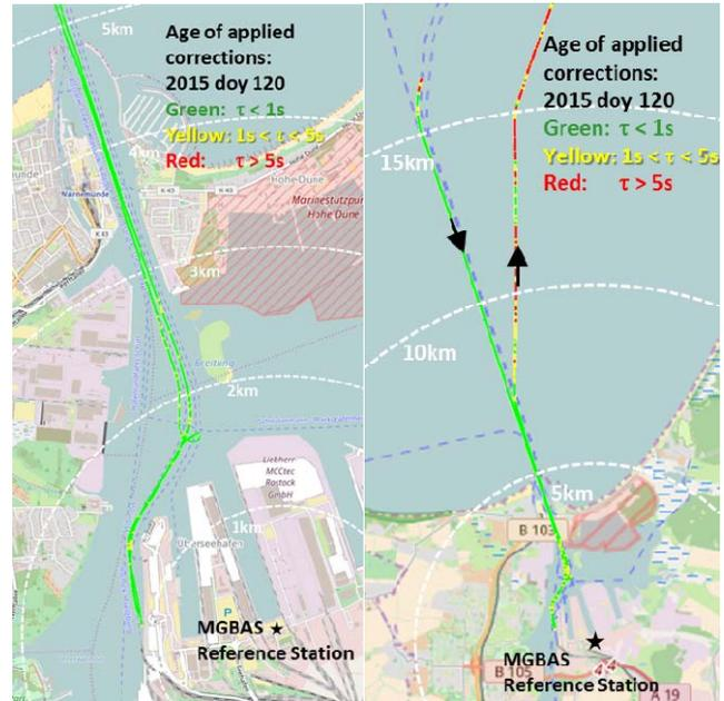
Figure 7. left - MGBAS data link availability with varying distance to the reference station; Age of applied corrections within data reception range (center) and within the service area of MGBAS in the port of Rostock (right)
