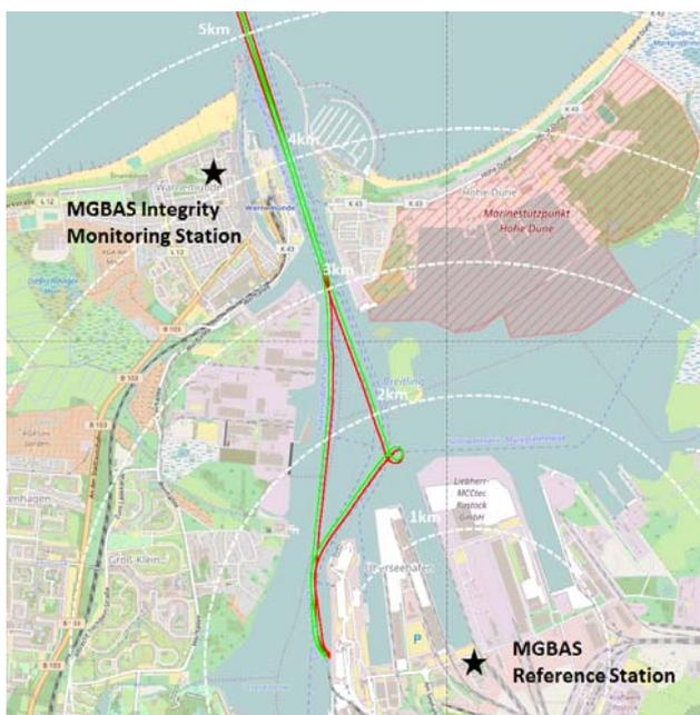
Figure 6. Vessel trajectory within the port of Rostock (green: starboard antenna, red: portside antenna), white dashed circles mark the distance to the MGBAS Reference Station
