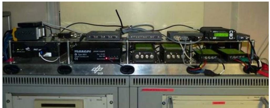
Figure 4: Left: Installation of starboard GNSS antenna with UHF antenna (right) for the reception of MGBAS correction data Right: Board with GNSS receivers, UHF modem, IALA Beacon receiver, serial to Ethernet adapter and Box PC for data processing and storage
