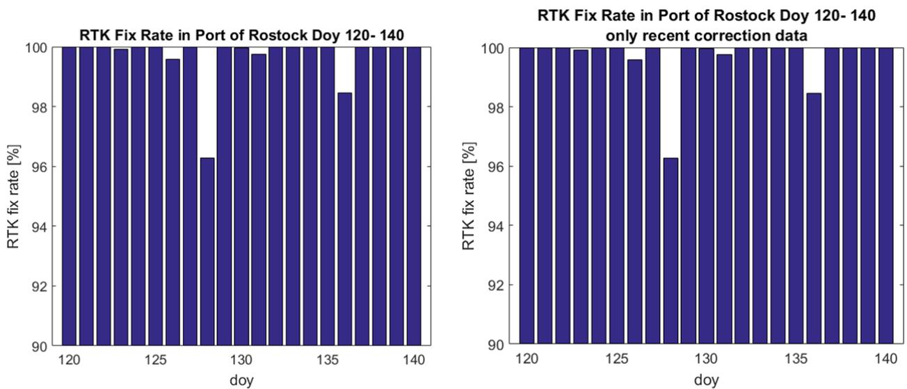
Figure 10. RTK Fix rate in the port of Rostock, left: using all data; right: using only recent correction data
