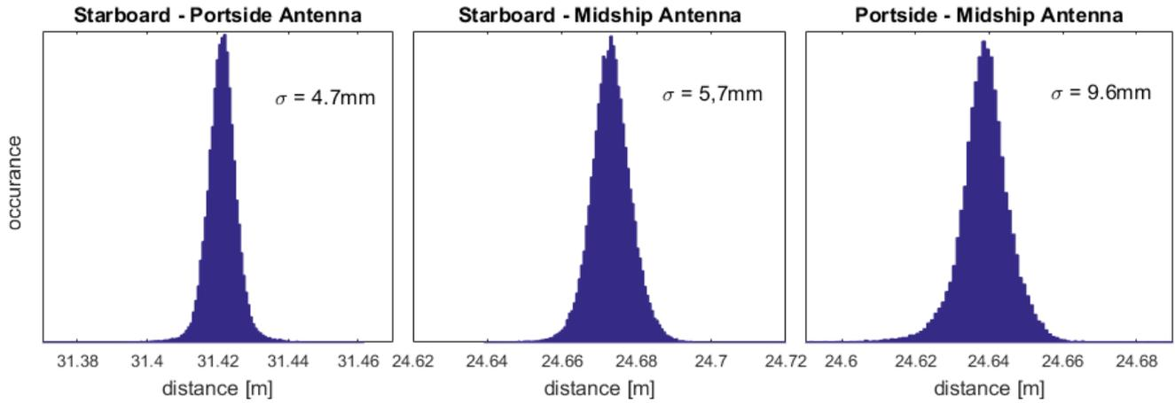
Figure 9. Histograms of calculated distances between the antennas based on RTK position results
