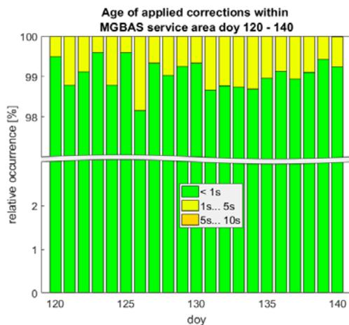
Figure 8. Age of applied correction for RTK positioning within service area of the MGBAS in the port of Rostock
