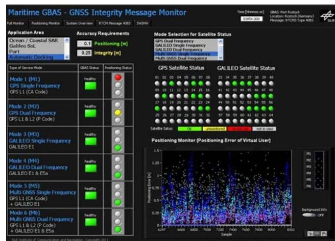
Figure 2. MGBAS Monitor for visualization of MGBAS relevant integrity statements
