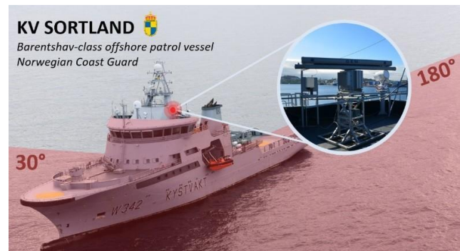
Figure 4. GEM GEMINI-DB radiation sector on KV SORTLAND offshore patrol vessel
