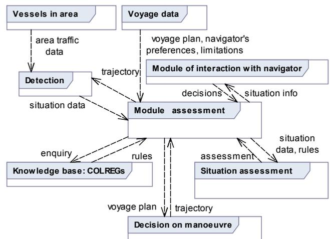
Fig. 1. Architecture of the navigational support system on a sea going vessel
