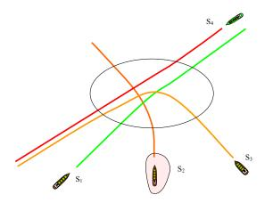
Fig. 2. Vessels that are likely to encounter within confined area create potentially dangerous situation
