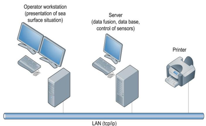
Figure 3. Functional diagram of the Control Centre.
