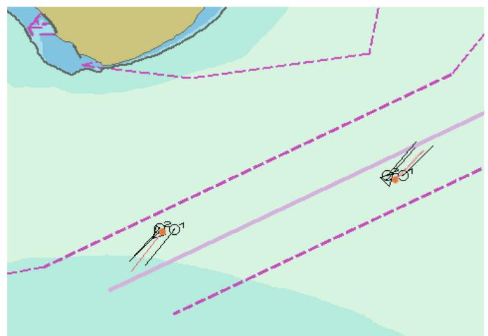
Figure 7. Two detected and tracked targets (circle 1 – FMCW radar, circle 2 – pulse radar, triangle – AIS, point – data fusion).
