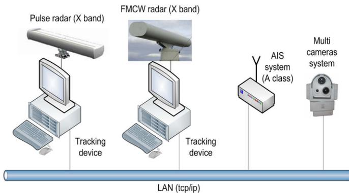
Figure 2. Functional diagram of the Observation Post.
