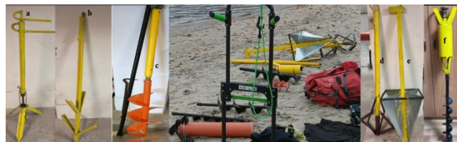
Figure 6. Prototypes of SAFL bottom anchors; a – prototype of 'Umbrella 1' anchor, b – prototype of 'Umbrella 2' anchor, c – initial prototype of 'SAFL Screw-In Anchor', d and e – prototypes of 'SAFL Flange Anchor', f – prototype of 'SAFL Screw-In Suction Anchor'. Source: Internal materials of Student Special Interest Group of Underwater Research 'SeaQuest' - January 2025.
