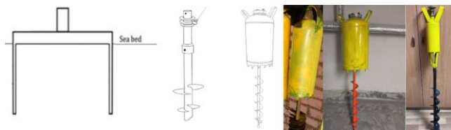
Figure 5. From left: 'Umbrella 1' SAFL, 'Umbrella 2' SAFL, SAFL Flange Anchor. Source: Internal Materials of the Student Special Interest Group of Underwater Research 'SeaQuest'.
