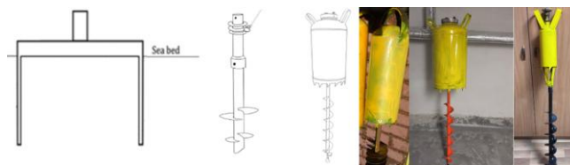
Figure 7. From left: Suction Caisson, Helix Anchor, SAFL Screw-In Suction Anchor prototypes. Source: Own study based on [4, 12, 13, 14], internal materials of Student Special Interest Group of Underwater Research SeaQuest.
