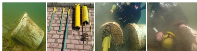
Figure 4. On the left, the first prototypes of SAFL bottom anchors anchored in the bottom of Lake Raduńskie in May 2024, used for mooring small watercraft at the Stella Maris center in Kashubia. On the right side is the old gravity anchor known as 'pig' (plastic bucket filled with concrete). Source: Internal materials of NKBP 'SeaQuest' – May 2024.
