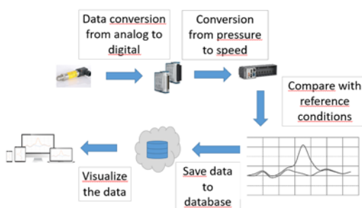
Figure 2. Online monitoring of thrust streams velocities over the seabed.
