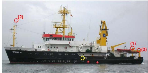
Figure 5. Vessel DENEK with sensor locations
