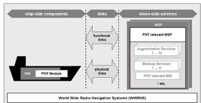
Figure 1. Generic architecture of the Integrated PNT System
