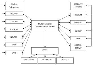
Figure 2. Multifunctional Communication System architecture.[11] [Own work].
