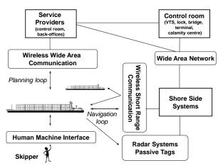
Figure 1.Structure of the date transmission in the RIS system. [12]
