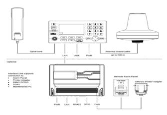
Figure 3. Integration architecture of the Iridium- Lars Thrane LT-3100S satellite segment module with the GMDSS in the Multifunctional Communication System. [16]
