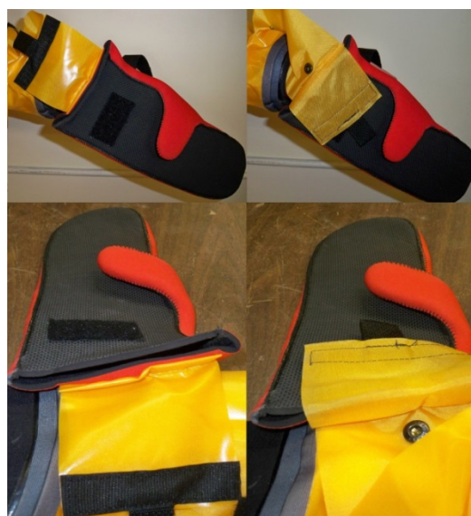
Figure 4. Design flaw: Inadvertent blocking of entrance into hand protection
