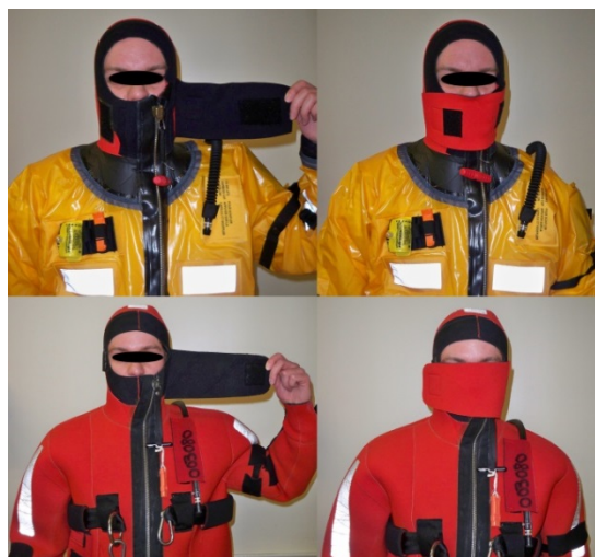
Figure 5. Comparison of Velcro male-female face shield attachment sites across the face
