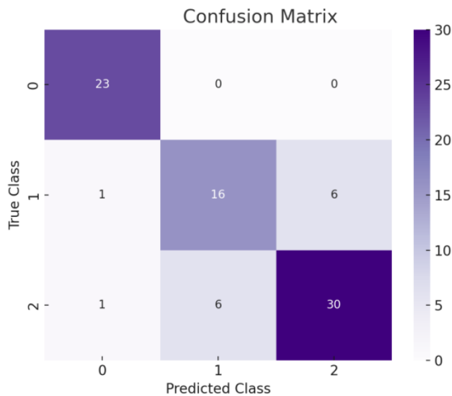
Figure 9. Confusion matrix showing the classification results of the cloud detection model. Class 0 represents cloud-free areas, class 1 corresponds to thin clouds, and class 2 refers to thick clouds.
