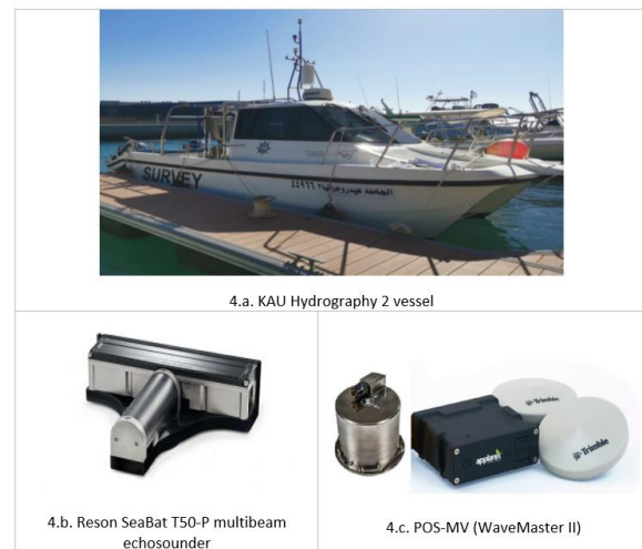
Figure 4. KAU Hydrography 2 vessel (4.a) along with Reson SeaBat T50-P multibeam echosounder (4.b) and POS-MV positioning and orientation system (4.c) [18][19].
