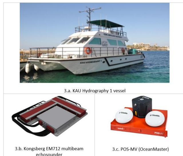
Figure 3. KAU Hydrography 1 vessel (3.a) along with Kongsberg EM712 multibeam echosounder (3.b) and POS-MV positioning and orientation system (3.c) [17][19]
