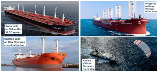
Figure 4. WASP installations on different types of ships. Source: Own research based on Source: Based on [24, 25, 26, 28].
