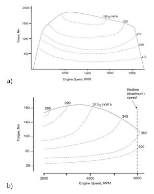
Figure 1. Typical operating map, showing lines of specific fuel consumption for: a) diesel engine; b) spark ignition engine
