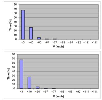
Figure 3. Garbage truck speed structure a) the truck equipped with CI engine b) the truck equipped with SI engine
