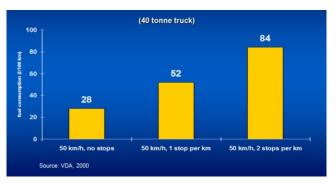
Figure 2. The influence of number of stops per 1 km on heavy truck fuel consumption
