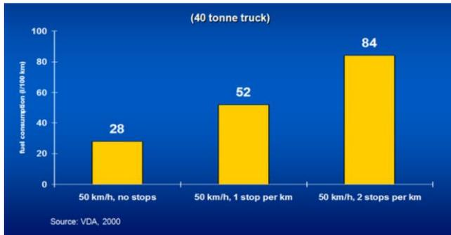
Figure 2. The influence of number of stops per 1 km on heavy truck fuel consumption
