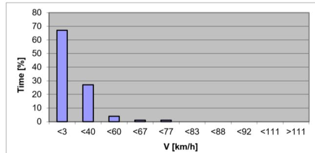
Figure 3. Garbage truck speed structure
