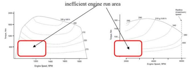
Figure 5. X1 Schematic engine map with inefficient engine run area
