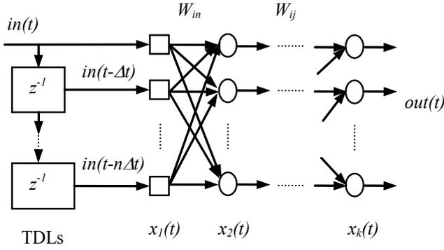
Figure 1. Neural network with feed-forward back-propagation (FFBP) architecture.
