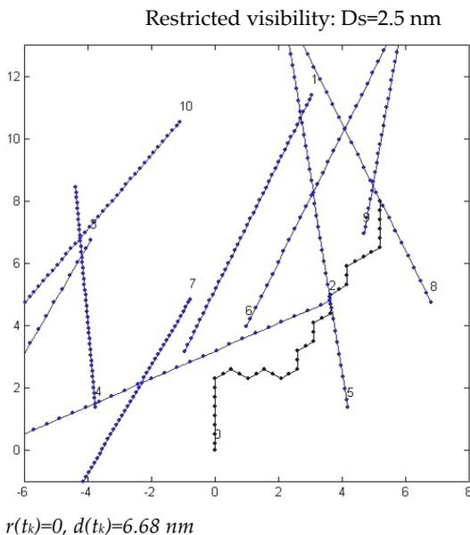
Figure 13. The ship's game trajectories for the GSC3 algorithm.
