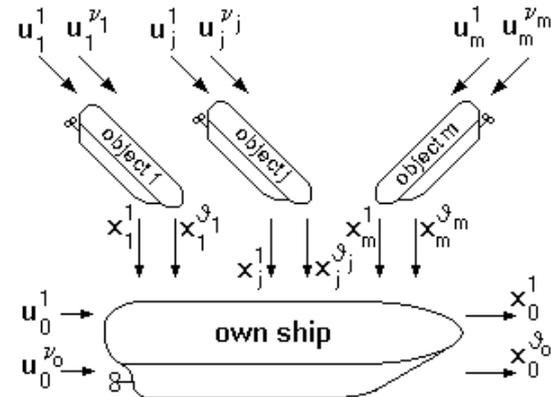
Figure 3. Block diagram of a model ship's differential game including  $j$  participants.
