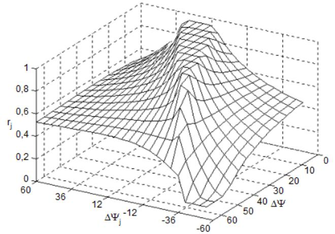
Figure 7c. Dependence of the collision risk on the strategy the own ship and that of the  $j$ -th encountered object to approaching from the stern.
