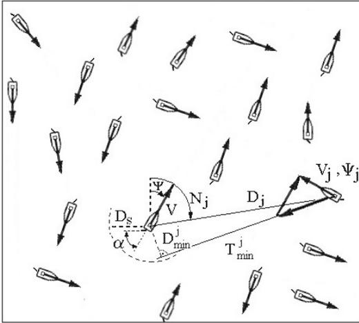
Figure 1. Parameters describing the process of the own ship passing  $j$ -th encountered ship.
