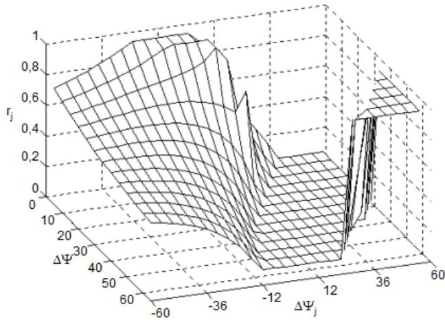
Figure 7a. Dependence of the collision risk on the strategy the own ship and that of the  $j$ -th encountered object to approaching from the LB.
