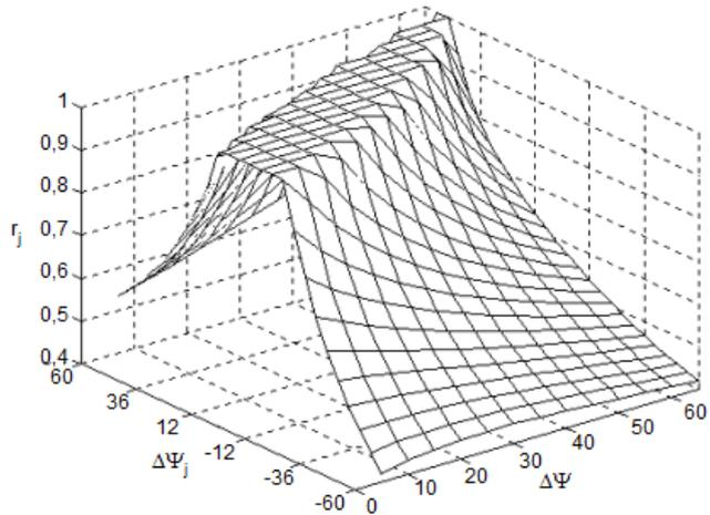
Figure 7b. Dependence of the collision risk on the strategy the own ship and that of the  $j$ -th encountered object to approaching from the SB.
