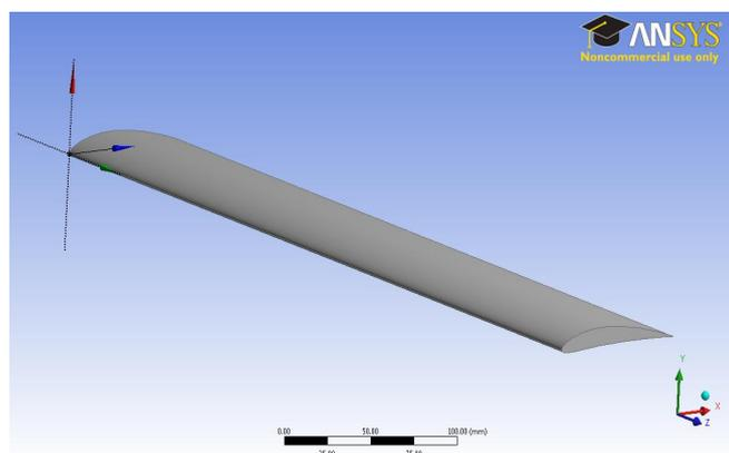
Figure 4 Geometric representation of the NACA 6412 profile
