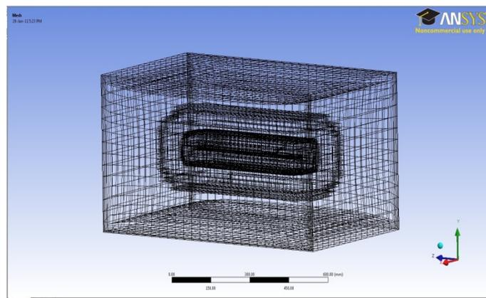
Figure 5. Profile discretization
