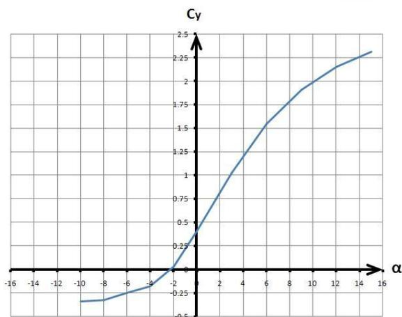
Figure 2. Graphic of  $C_y$  experimentally obtained
