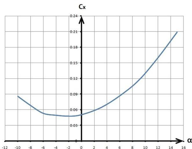
Figure 7. Graphic of  $C_x$  obtained using CFD
