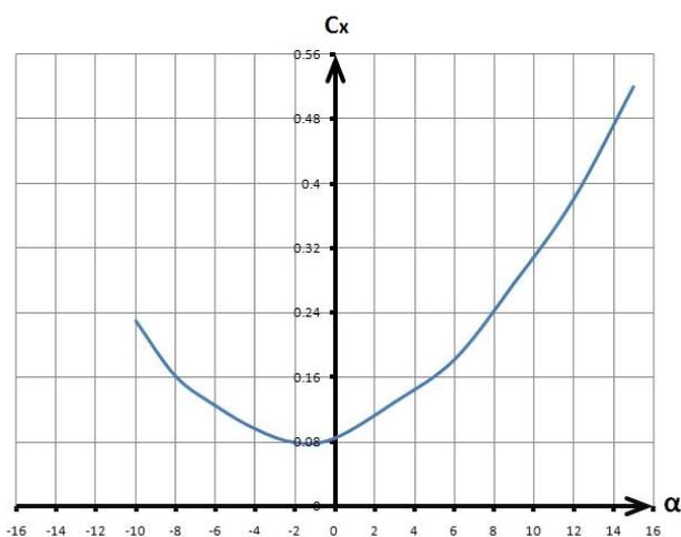
Figure 3. Graphic of  $C_x$  experimentally obtained
