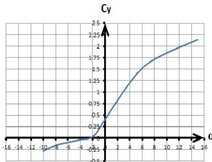
Figure 6. Graphic of  $C_y$  obtained using CFD
