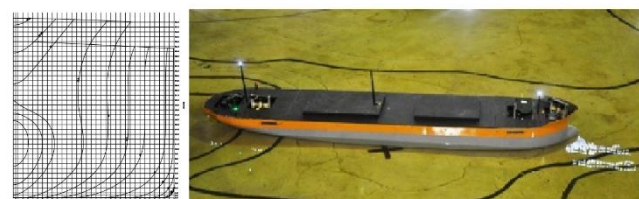
Figure 2. Body plan of the full-scale ship (left) and the corresponding scale model built in fiberglass (right).
