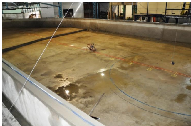
Figure 1. Physical model at the USP used for reduced-scale manoeuvring tests.
