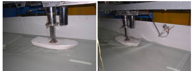
Figure 6. Dhow model test in vicinity of vertical wall, Left moderate speed, Right high speed
