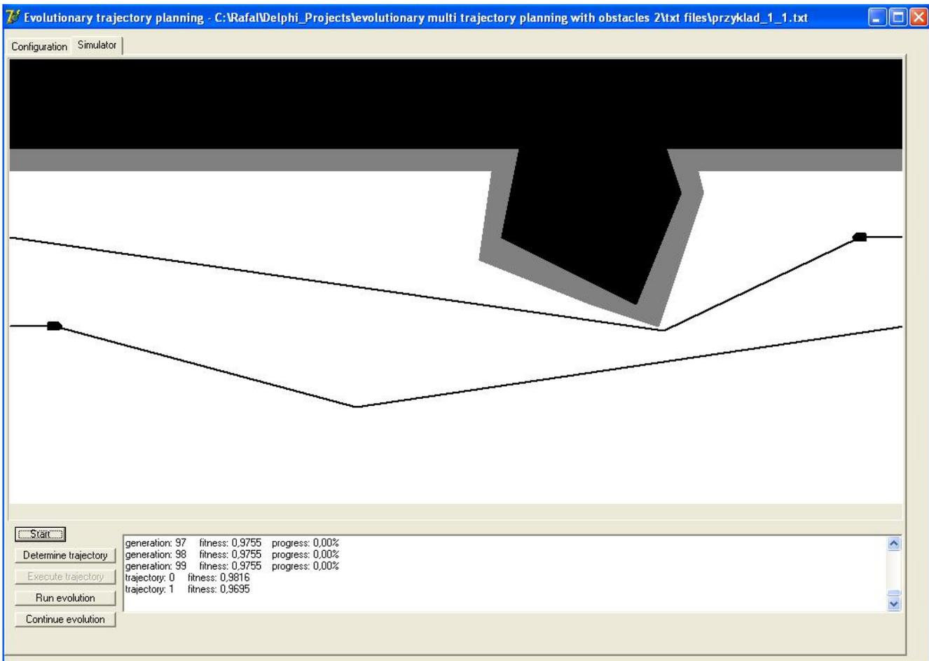
Figure 15 The evolutionary set of the two ships' cooperating trajectories, which avoid collisions with the landmass and each other.
