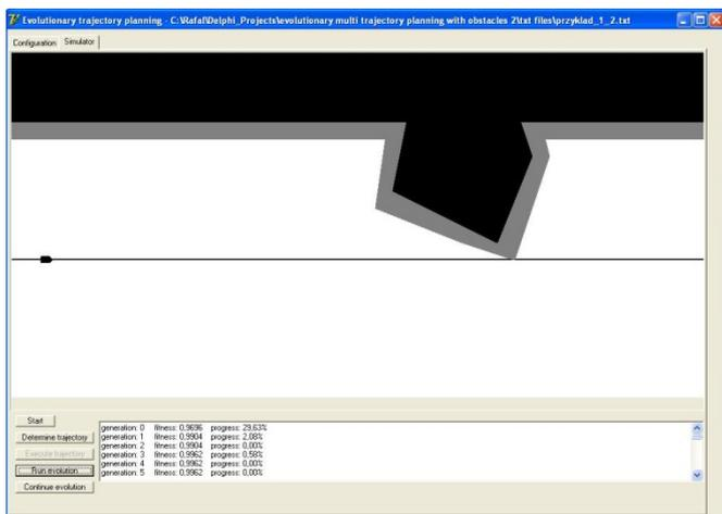
Figure 12 The own ship's current course does not collide with the landmass (black) or its domain (grey).
