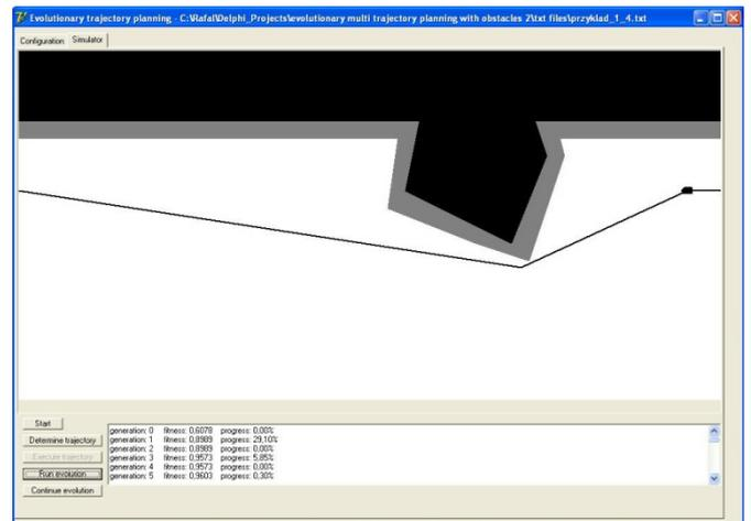
Figure 14 The target's current course collides with the landmass so the target will perform a collision avoidance manoeuvre.
