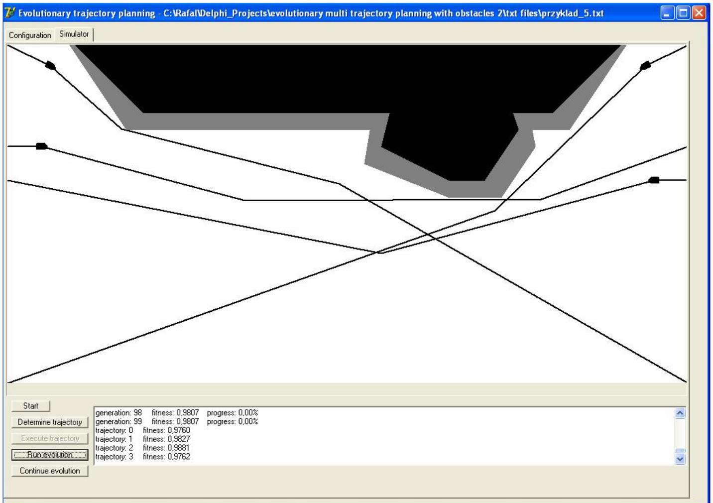
Figure 21 The evolutionary set of the four ships' cooperating trajectories, which avoid collisions with each other and the landmass (landmass in black, landmass domain in grey).
