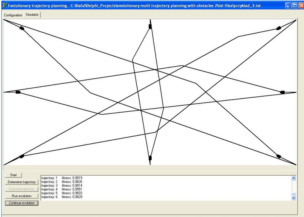
Figure 20 The evolutionary set of the eight ships' cooperating trajectories, which avoid collisions with each other.
