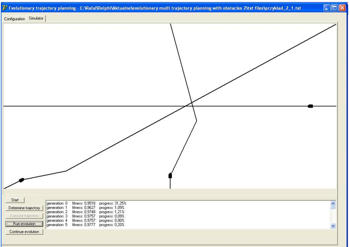
Figure 19 The evolutionary set of the three ships cooperating trajectories, which avoid collisions with each other.
