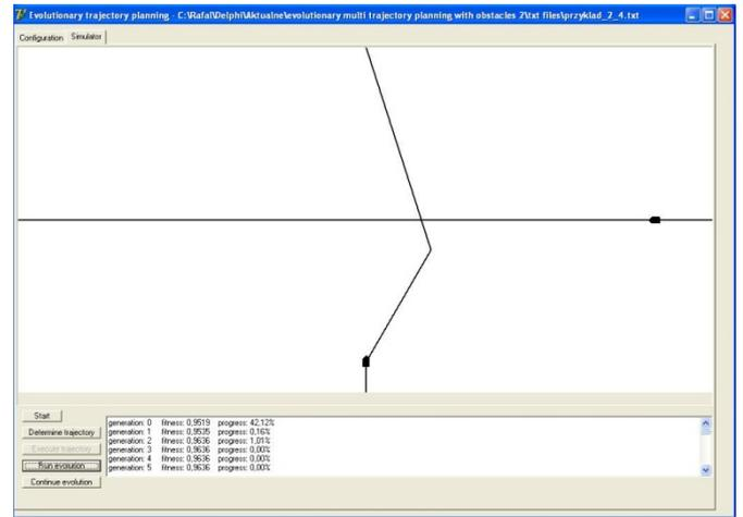
Figure 18 The first target's current course (left) collides with target 2 (right) and target 1 performs collision avoidance manoeuvre.
