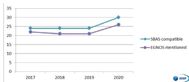
Figure 2. SBAS compatible device evolution in SOLAS satellite navigation equipment
