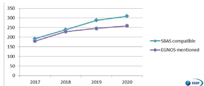
Figure 5. SBAS compatible device evolution in non-SOLAS satellite navigation equipment
