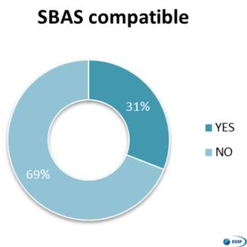
Figure 12: Percentage of SBAS compatible devices within AIS non-SOLAS equipment
