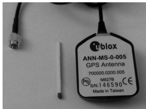
Figure 2. u-blox GPS Antenna with magnetic base.
