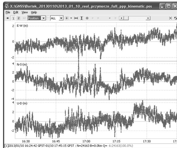
Figure 18. The results of PPP-kinematic positioning in combined mode.
