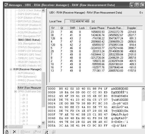
Figure 8. Sample UBX\RXM\RAW frame from the u-center.
