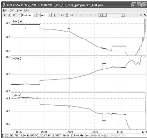
Figure 15. Static positioning in backward positioning mode.
