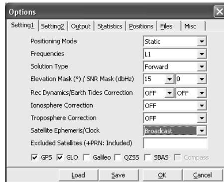
Figure 12. RTKLIB algorithm configuration - the major part.
