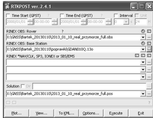
Figure 11. Configuration of the RTKLIB input files.
