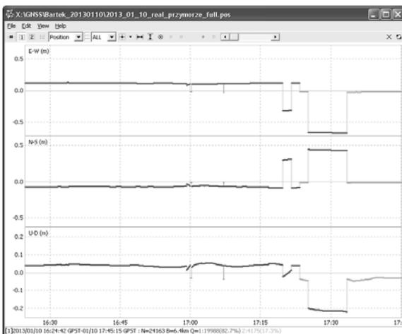
Figure 16. Static positioning in combined positioning mode.
