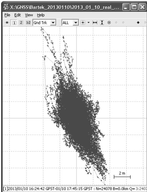
Figure 9. The result of single solution positioning.
