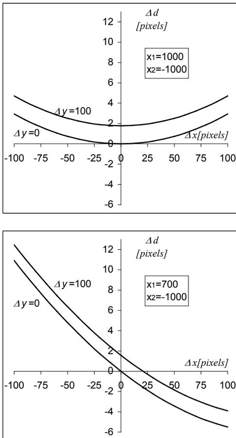
Fig. 9. Error  $\Delta d$  of angular distance resulting from shifting of focus about values  $\Delta x$  and  $\Delta y$  in relation to middle of array; for symmetrical (upper) and asymmetrical (lower) measurements.
