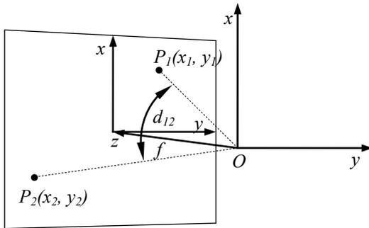
Fig. 1. Association of image sensor array with coordinate system  $Oxyz$  set by main plane of objective  $Oxy$  and its optical axis  $Oz$
