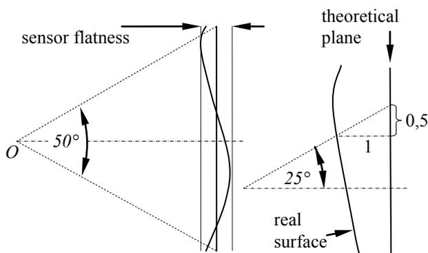
Fig. 4. Inaccuracy of arrangement of pixels at one plane
