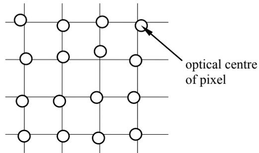
Fig. 2. Inaccuracy of placing of pixels optical centers on nodes of virtual net with equal mesh
