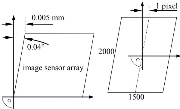
Fig. 3. Non-perpendicular pixels arrangement on image sensor array
