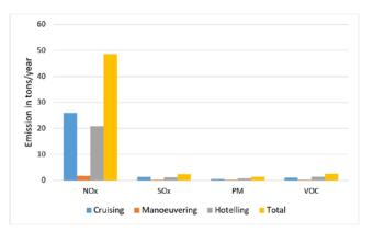
Figure 4. Cargo ship emissions in 2018 for each activity
