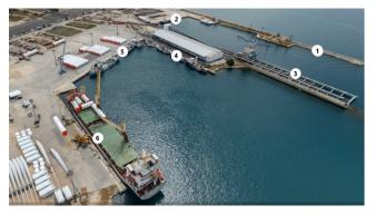
Figure 2. Cargo Port of Zadar: 1 – terminal for liquid cargo, 2 – oil platform supply terminal, 3 – terminal for bulk carriers, 4 – terminal for general cargo, 5 and 6 – terminal for general cargo and cement
