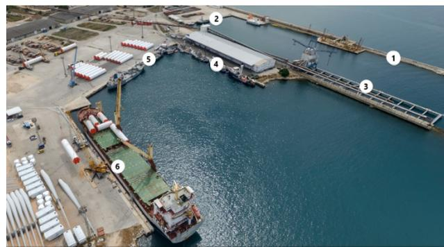
Figure 2. Cargo Port of Zadar: 1 – terminal for liquid cargo, 2 – oil platform supply terminal, 3 – terminal for bulk carriers, 4 – terminal for general cargo, 5 and 6 – terminal for general cargo and cement
