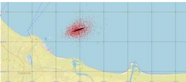
Figure 8. Oil spot moved due to the wind with uncertainty factor - GNOME. [2]
