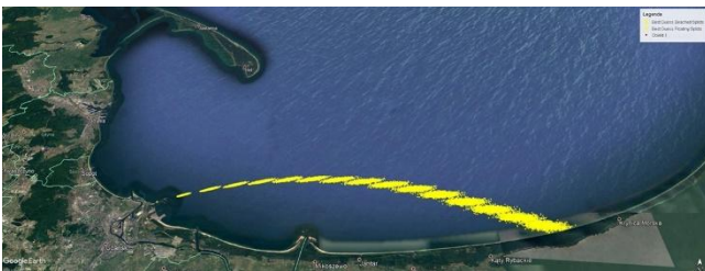
Figure 7. Trajectory of oil spill with interval every 4 hr - Google Earth.
