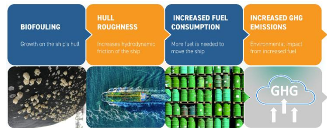
Figure 2. The ship hull biofouling [5]
