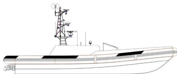
Figure 2. General Arrangement of a high-speed maritime vessel - a Search and Rescue (SAR) craft. These types of vessels are typically designed for rapid response to emergencies at sea and equipped with advanced intelligent navigation and communication systems to perform rescue operations.
