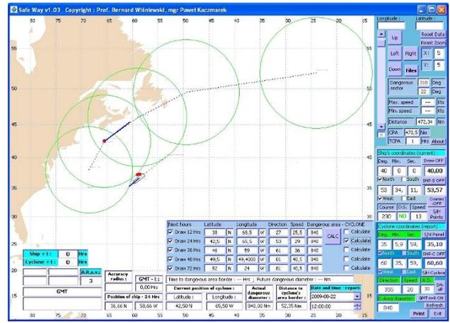
Figure 8 Graphic picture of cyclone and ship D positions according to the message on 22-08-2009, after altering course.
