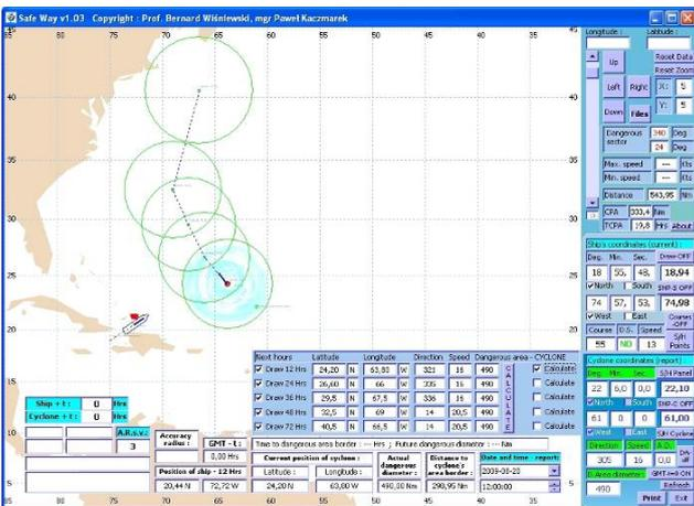
Figure 6 Graphic picture of cyclone and ship C positions during the voyage and calculation results.
