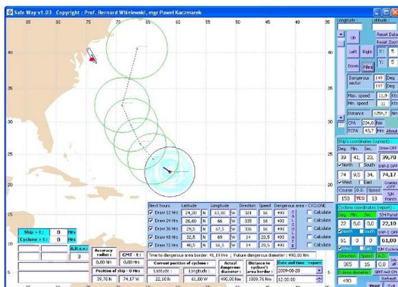
Figure 1 Graphic illustration of the cyclone path, based on weather report and calculations for ship A, heading for Brazil (20-08-2009, 12.00UTC).
