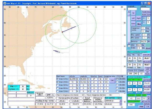
Figure 9 Graphic picture of cyclone and ship D positions after 12 hours after altering course to 288 degrees, voyage to New York.
