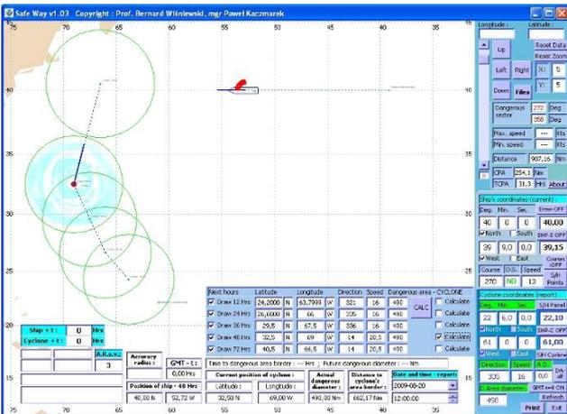
Figure 7 Graphic results of cyclone track according to message and calculation results for ship D after 48 travel hours from 20-08-2009, at 1200 UTC.
