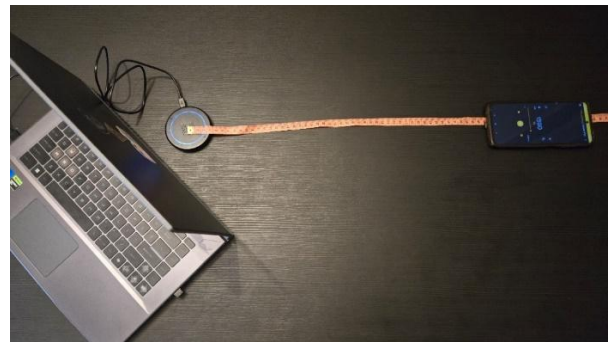
Figure 6. Laboratory setup view (laptop, microphone array, and phone as the acoustic signal generator).
