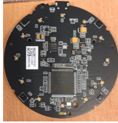
Figure 5. The ReSpeaker USB Mic Array device with the four microphones labelled
